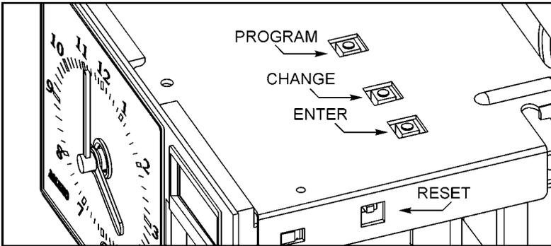
The **PROGRAM** button is used to enter and exit the Program Mode. Press the PROGRAM button at any time to exit the Program Mode. If a program step is in the process of being changed when this button is pushed, the new information will not be saved.
