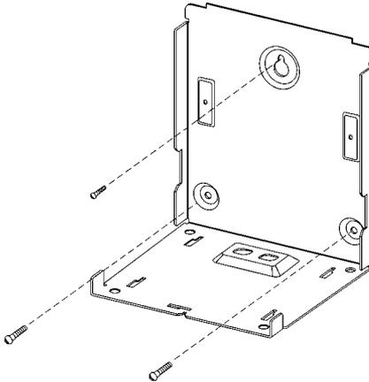
4. Approximate the final location of the clock. Insert one #10 wood screw or equivalent into the wall 1-1/2" (38 mm) from the top center location of the clock.
